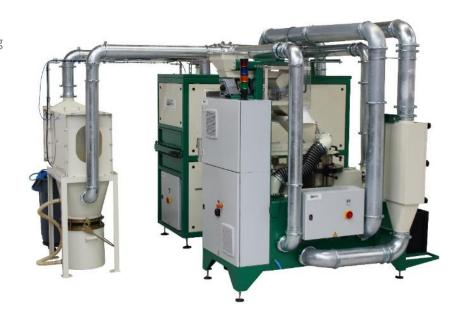
Testing was conducted using Seed Processing Holland's FDM Rotary Dryer Coater across a range of crop types, including oilseed rape (OSR), sunflower, and maize.
